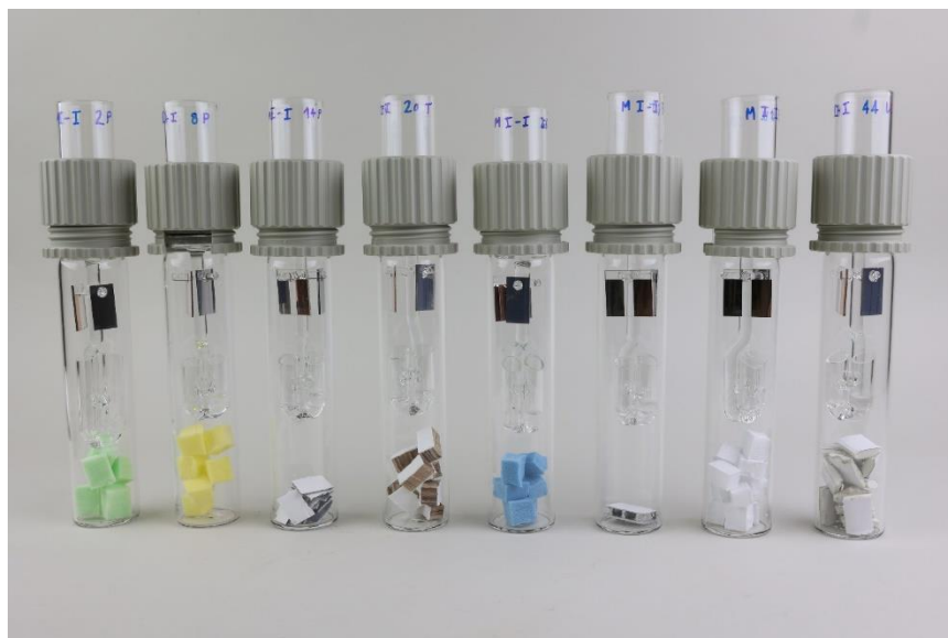
Figure: Validation of indicators using foams and boards as test material
