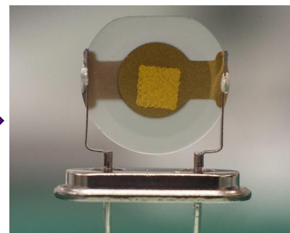
Figure 3: Piezoelectric quartz crystal before and after printing a mastic resin coating.
