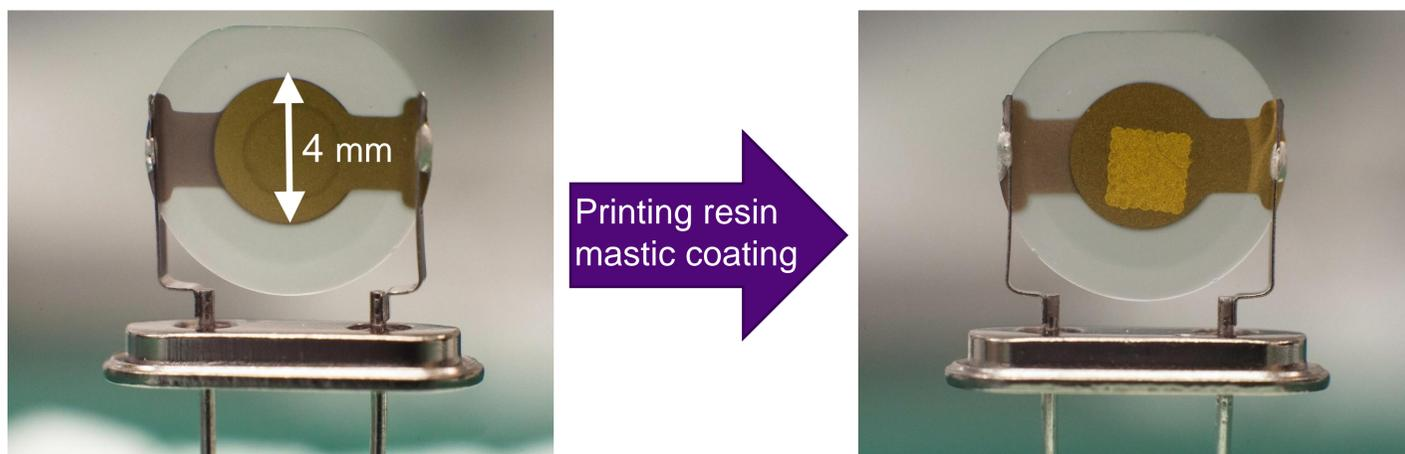
Figure 3: Piezoelectric quartz crystal before and after printing a mastic resin coating.
