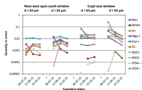
Ion chromatography of a series of dust samples in nave and crypt.
