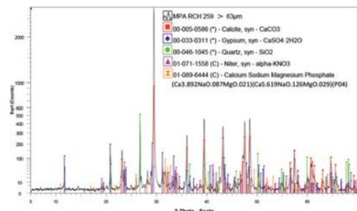
Example of x-ray diffraction of dust samples.
