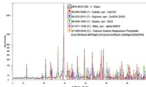
Example of x-ray diffraction of dust samples.
