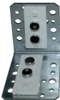
Passive sampling device with boron and carbon pads.
