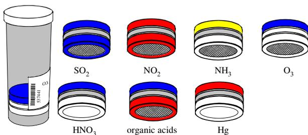
Samplers are marked with different colours depending on the gas and the sample is identified by a barcode.
