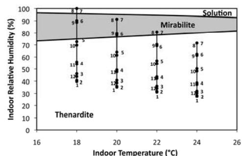
Figure 2: Indoor cycles for a building in Rome whose temperature is kept constant at 18°, 20°, 22°, 24°C respectively, for the local monthly T and RH averages in the 1961-1990 reference period. Humidity Mixing Ratio and numbered labels as in figure 1.
