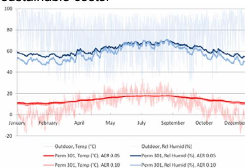
Figure 1: The simulated climate in the fully loaded permanent storage room at the air exchange rate 0.05 per hour and 0.1 per hour; in the background the monitored outdoor conditions [1].
