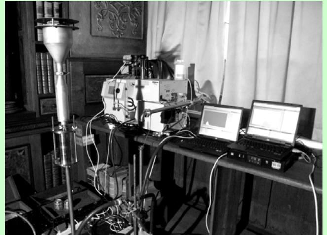
Scanning Mobility Particle Sizer (left) with next Aerodynamic Particle Sizer standing on Condensation Particle Counter, © Smolik
