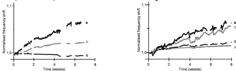
Figure 1: (left) Response of piezoelectric dosimeters exposed in the Exhibition (a) and in the Storage Room (b) of the HM and in the Control Chamber (c). (right) Response of piezoelectric dosimeters exposed in the Exhibition Rooms of the HM (a) and of the AM (b) and in the Storage Rooms (c and d, respectively).
