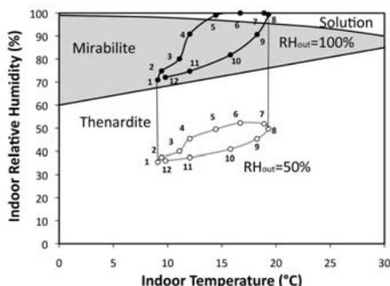
Figure 1: Thenardite-Mirabilite transformations outdoors and in an unheated historical building in Paris, calculated for outdoor RH=50 and 100%. Indoor Humidity Mixing Ratio is supposed to be as outdoors. Numbered labels indicate the calendar months.
