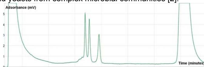
Figure 1: DHPLC chromatogram of a mixture of three fungi extracted and amplified. Conditions: DNASep Cartridge 0.9mL/min, wave optimized buffers A and B, gradient 59% at 57°C.
