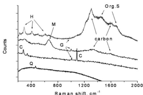
Figure 1: Raman spectra of the single particles. H – haematite, M- magnetite, Q – quartz, C – calcite, G - gypsum, Org.S. – organic substances.
