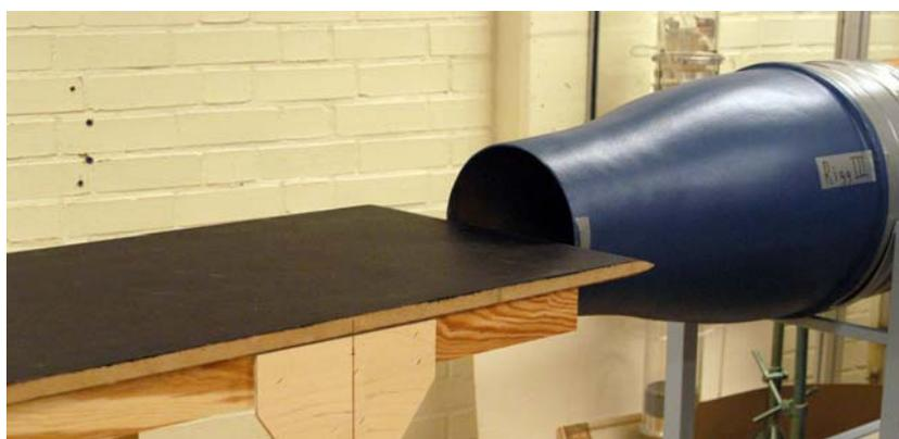
Figure 1: Left; the table where the samples were placed. Right; the nozzle from which air was blown over the plastered surfaces.
