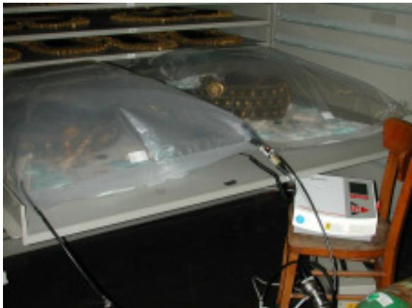
**Figure 1.** Checking the gas mixture within a package.
