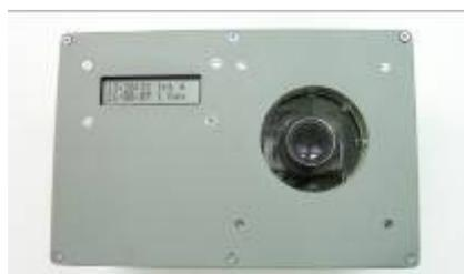
**Figure 1.** Prototype particulate deposition monitor.
