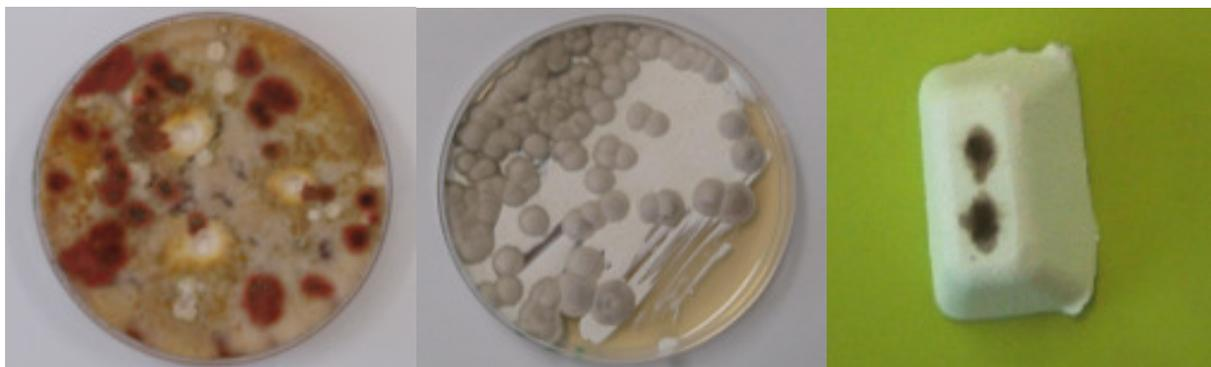
**Figure 1.** Agar diffusion test with *Epicoccum nigrum*; paint containing nano-silver particles with colonies of *Cladosporium cucumericum*; cement cube covered with nano-silver coating and inoculated with *Alternaria alternata*.
