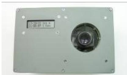
**Figure 1.** Prototype particulate deposition monitor.
