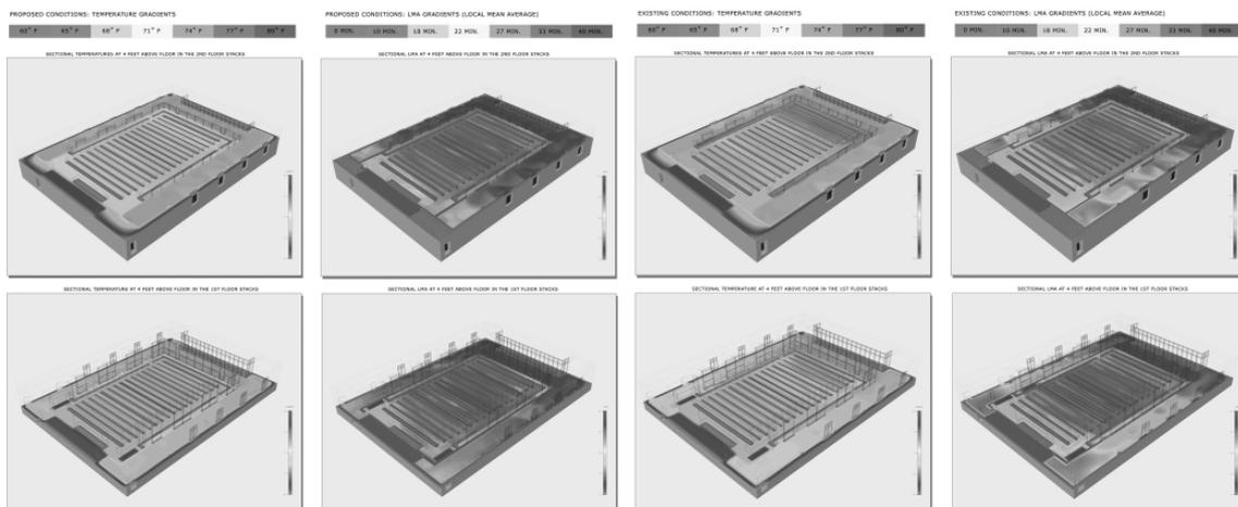
**Figure 1.** Computer simulation results of air temperature and local mean age of air.
