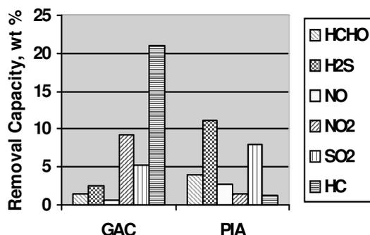
Figure 1. Removal capacity of GAC vs. PIA.
