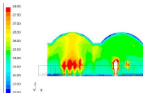
**Figure 2.** Results of simulation; distribution of air temperatures.
