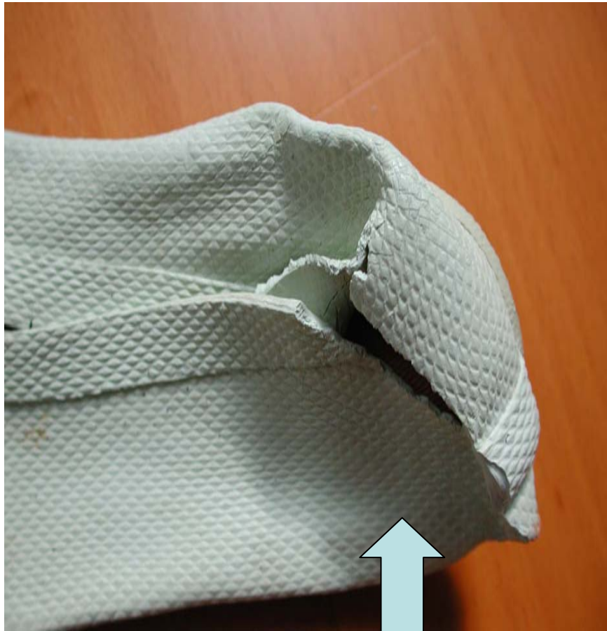
Stiff, oxidized rubber shoe
