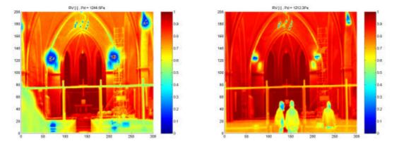
*Relative humidity near the surface as calculated from absolute humidity and thermographic surface temperatures; during 2 hours of open air gas heating (left), directly after heating (right)*
