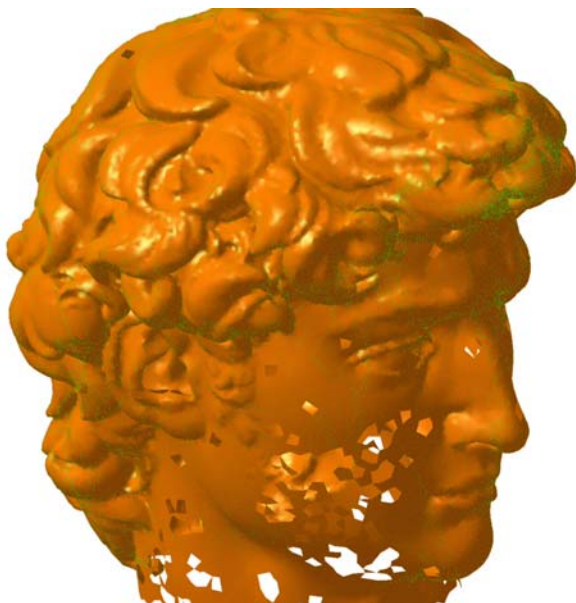
Fig.3 - The cloud of points tassellated contains holes that have to be manually filled
