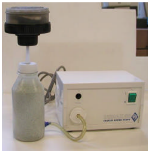
Figure 4b Filter pump for removing reduced sulphur gases
