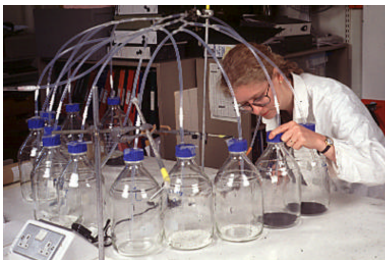
Figure 3a Experimental apparatus for evaluating adsorbents for reduced sulphur gases.
