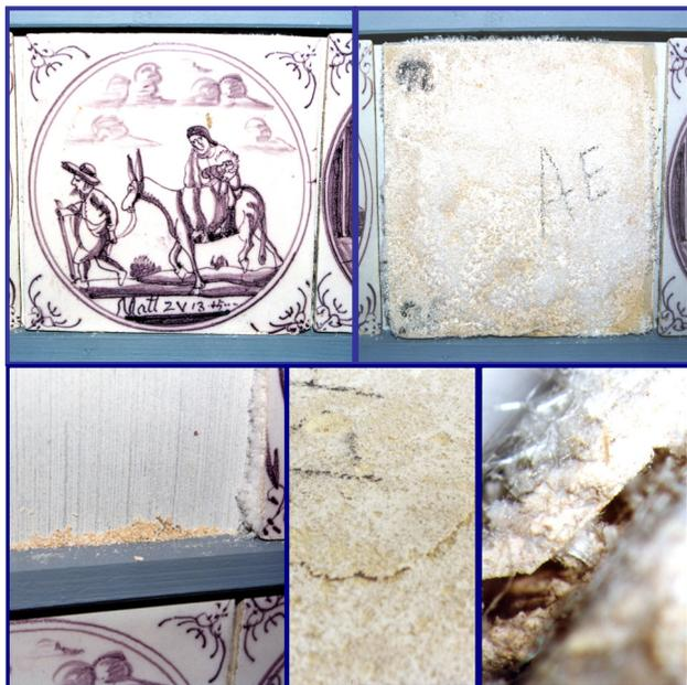
Fig. 1 Dutch tin glazed tiles (18<sup>th</sup> century) in display case: efflorescences and damage.
