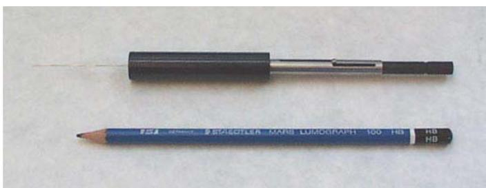
**Figure 1: The SPME holder with the fiber exposed (left).
