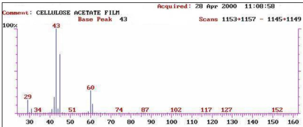
**Figure 4: Mass spectrum of the acetic acid peak from a cellulose acetate negative emission test. Together with the retention time from the GC chromatogram, a mass spectrum gives a high confidence in identification of compounds**
