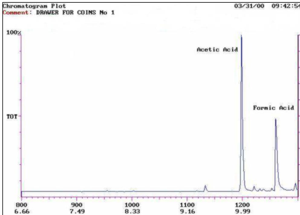
Figure 3: Chromatogram of emission from the wooden drawer. The acetic acid emission was measured quantitatively but a formic acid peak is also visible.
