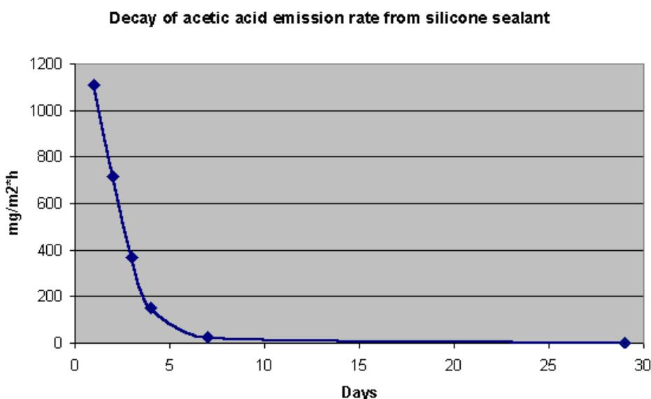
**Figure 5: Emission profile of Bostik 2680 silicone sealant over 29 days.**
