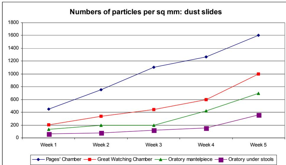
Consistently more particles are seen on the dust slides than on the sticky pads, and their average size is smaller. As explained above, this is because of the difficulty in discriminating small and dark-coloured particles against a black background. The end result is that the area covered as estimated from the slides is about 20% greater than that estimated from the sticky pads.
