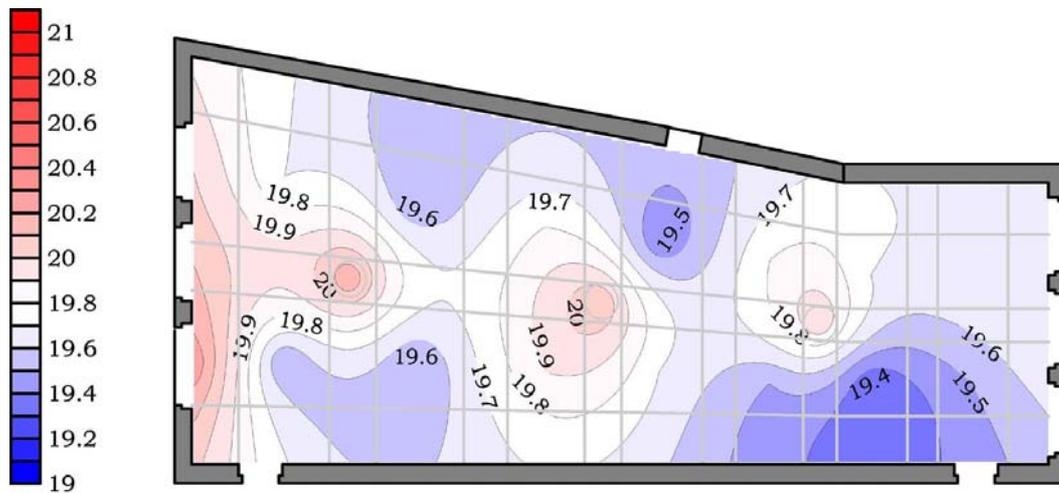
Figure 2: Wooden ceiling temperature (°C) with hot spots determined by three chandeliers with 20 compact fluorescent lamps. Hall of Giants, Padova (I), measurements taken in the occasion of a concert.
