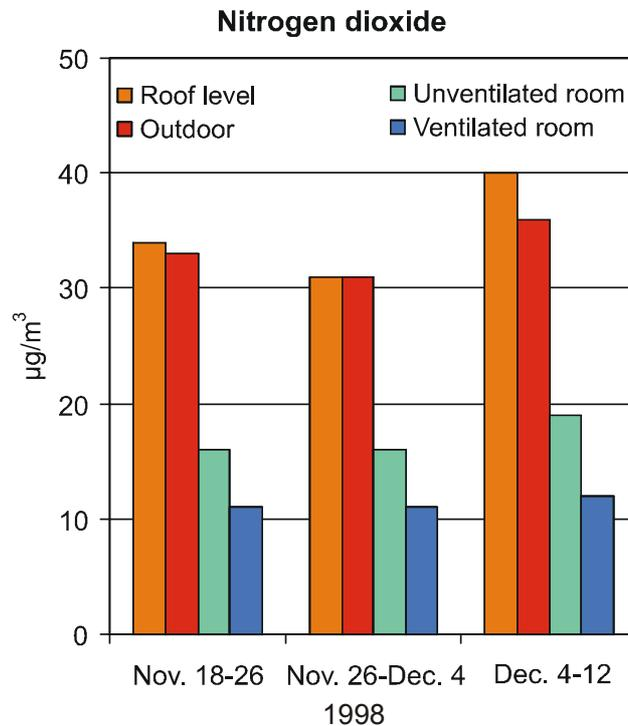
**Figure 3: Nitrogen dioxide measured in the two rooms compared to two outdoor locations**
