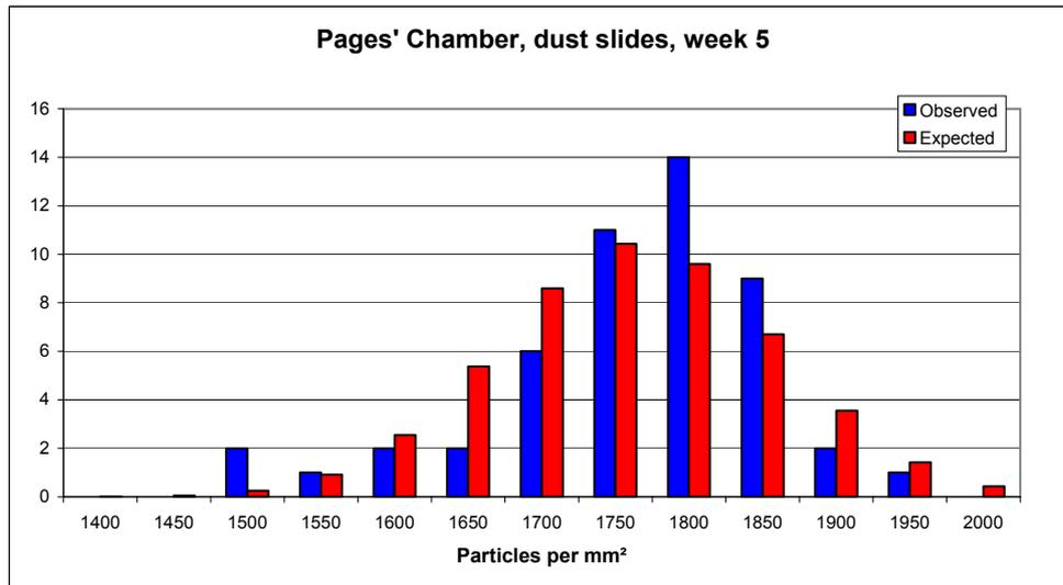
The results for both numbers of particles per square millimetre and total area covered show a reasonably good fit to a Gaussian distribution calculated using the means and standard deviations obtained from the data. The fit is not perfect, but nevertheless it is good enough to be able to say that both numbers and areas do follow Gaussian statistics.
