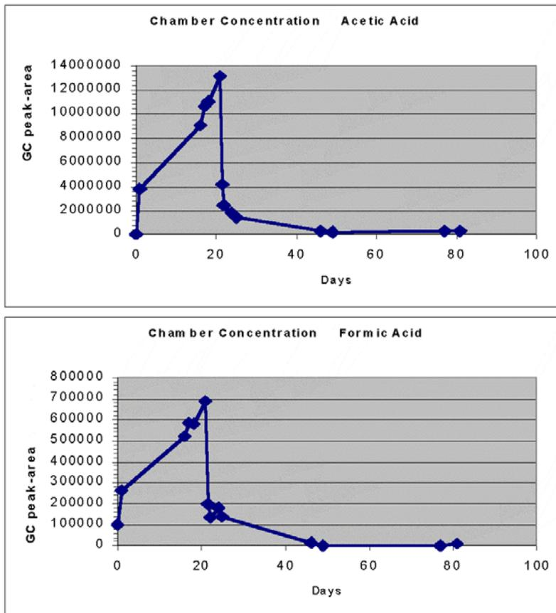
Figure 4: Decay curves for acetic acid (top) and formic acid (bottom) concentrations over 80 days in the chamber set-up. The lead foil was inserted on day 21.
