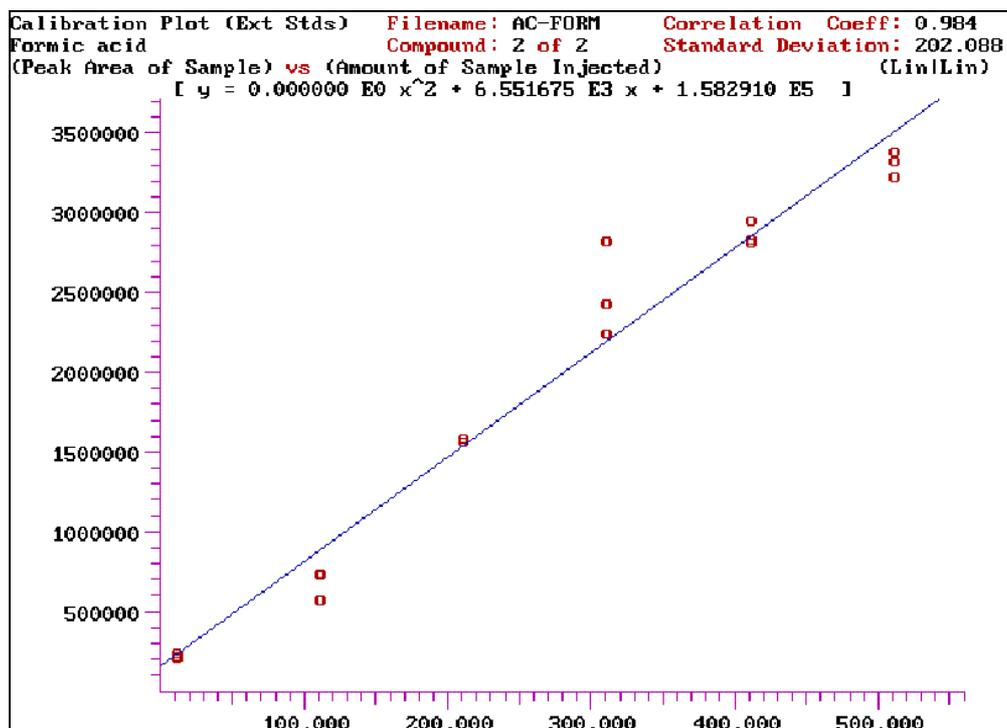
Figure 2: Calibration curve, formic acid
