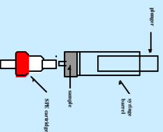
Figure 1 : A schematic diagram of the SPE apparatus.
