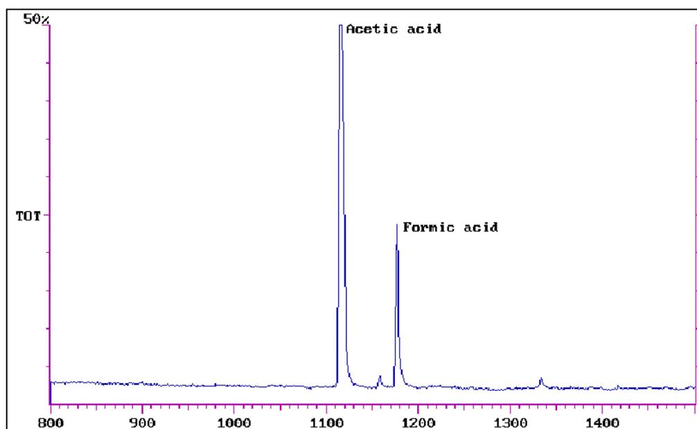
Figure 1: Chromatogram of acetic and formic acid in air, sampled on SPME (PA 85 $\mu$ )
