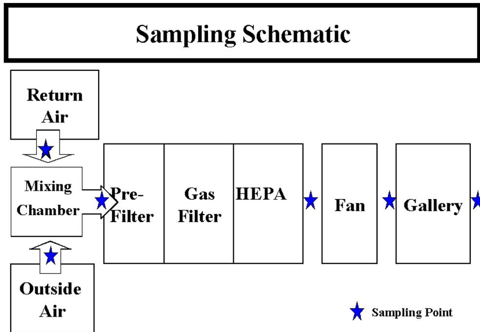
Figure 1: Schematic diagram of measuring sites, upstream and downstream from filter bank
