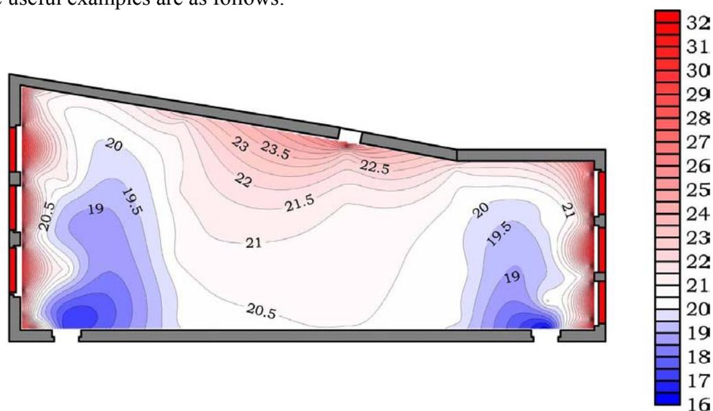
Figure 1: Floor temperature (°C) with cold areas in front of two open doors determined by the entrance of air from the nearby cooler corridor. Room heating is made with radiators (red rectangles on the shorter sides) and floor heating. Hall of Giants, Padova (I), measurements taken in the occasion of a concert.
