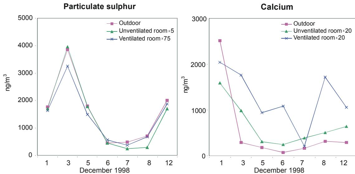
**Figure 2:** Time series for the total concentration of “anthropogenic” particulate sulphur and the “soil” element calcium.
