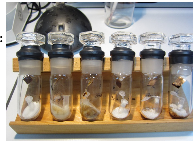
metal coupons on nylon filament hanging freely above standard A and B
