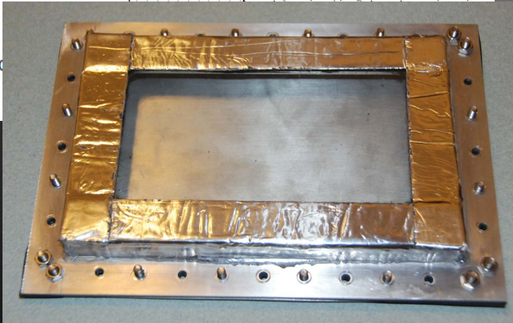
A prototype A5 size anoxic frame for use in a Suntest XPS+ chamber
