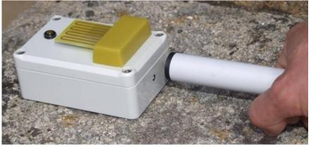
Corrosion depth =  $t_{init} \left( 1 - \frac{R_{ref}}{R_{sens}} \frac{R_{sens,init}}{R_{ref,init}} \right)$
