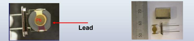
The PQC-dosimeter responds to the cumulative dose received and can be responsive to (1) volatile organic acids or (2) photooxidising effects.
