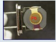
Change (%) is calculated from the frequency shift  $\Delta f(Hz)$  relative to the original frequency of the crystal (*Fo(kHz*) after coating
