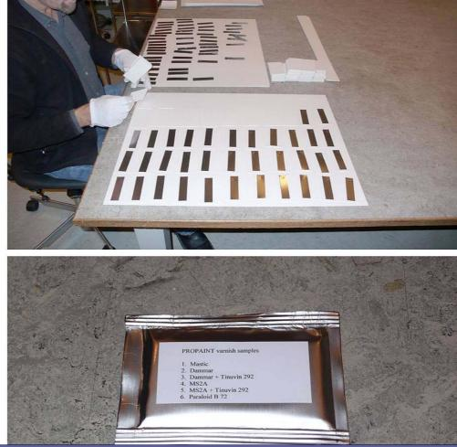
Varnishes selected **1.Resin Mastic** 2.Dammar 3.Dammar and Tinuvin 4.MS2A 5.MS2A and Tinuvin 6. B72
