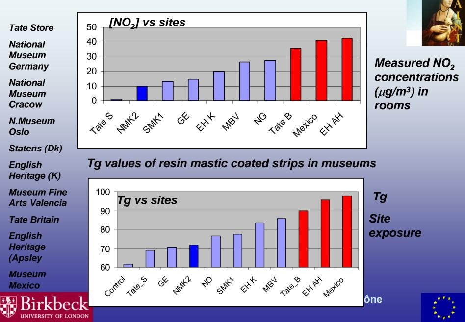
Resin Mastic Tg of strips in museums within frames (F) and in rooms (R) and measured  $NO_2$ ,  $O_3$ , HAc values in frames and in rooms
