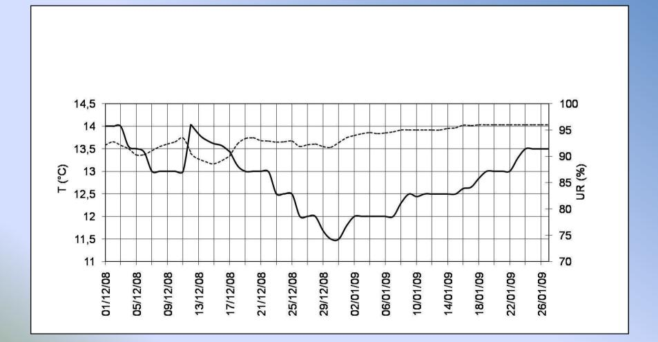
Temperature (T-continue line) & Relative Humidity (UR-dotted line) monitoring in spring
