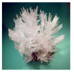
Mirabilite exerts a very high crystallization pressure on the pore wall causing damage of the stone. Moreover, the transient stress can remain for a long period of time since the relaxation process is slow (Espinosa et al., 2008).
