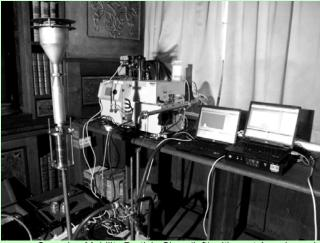
Scanning Mobility Particle Sizer (left) with next Aerodynamic Particle Sizer standing on Condensation Particle Counter,© Smolik
