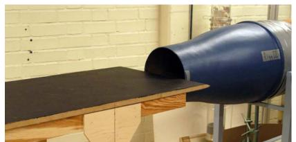
Figure 1: Left; the table where the samples were placed. Right; the nozzle from which air was blown over the plastered surfaces.
