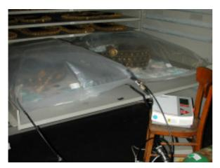
Figure 1. Checking the gas mixture within a package.
