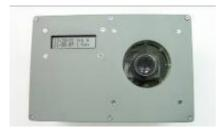
Figure 1. Prototype particulate deposition monitor.
