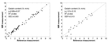
**Figure 1.** PLS calibration for prediction of gelatin content in historic paper: the developed model (left) and external validation (right).
