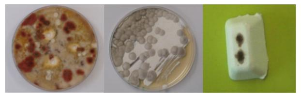
Figure 1. Agar diffusion test with *Epicoccum nigrum*; paint containing nano-silver particles with colonies of *Cladosporium cucumericum*; cement cube covered with nano-silver coating and inoculted with *Alternaria alternata*.
