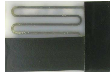
Zinc sensor / electrodeposition / about 2 μm
