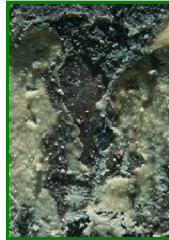
Microscope view of glass surface attacked by air pollution
