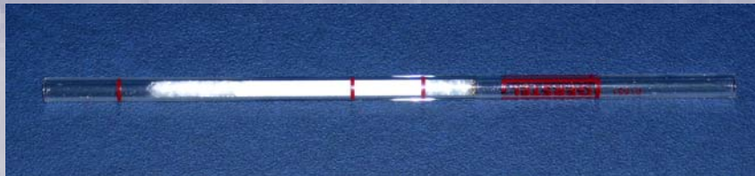
Tenax TA tube (200 mg, 60-80 mesh)
