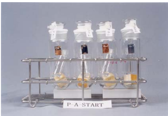
Photo 4. P-A test tube of Oddy test
