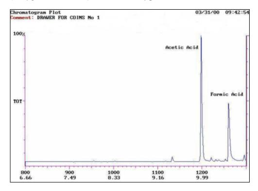
Figure 3: Chromatogram of emission from the wooden drawer. The acetic acid emission was measured quantitatively but a formic acid peak is also visible.
