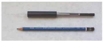
Figure 1: The SPME holder with the fiber exposed (left). The size can be compared with the pencil. Sampling is performed by exposing the fiber to the air leaving the chamber. Analysis of collected components was performed by gas chromatography/mass spectroscopy (GC/MS) using the injector to desorb the components collected. No organic solvents are used during analysis, and the time used from start of sampling to analysis results is 35 minutes.
