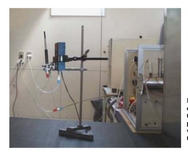
Figure 2: The sampling setup, connected to the chamber by teflon tubings. The SPME fibre is in position ready for sampling, at the white Omnifit teflon holder next to the pump.
