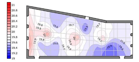
Figure 2: Wooden ceiling temperature (°C) with hot spots determined by three chandeliers with 20 compact fluorescent lamps. Hall of Giants, Padova (I), measurements taken in the occasion of a concert.
