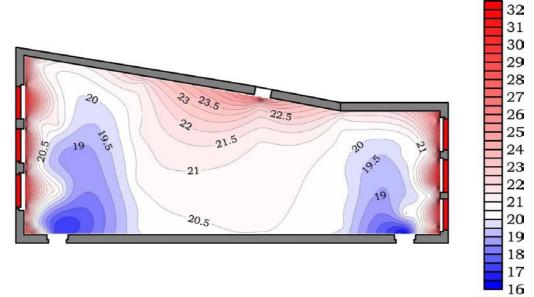
Figure 1: Floor temperature (°C) with cold areas in front of two open doors determined by the entrance of air from the nearby cooler corridor. Room heating is made with radiators (red rectangles on the shorter sides) and floor heating. Hall of Giants, Padova (I), measurements taken in the occasion of a concert.
