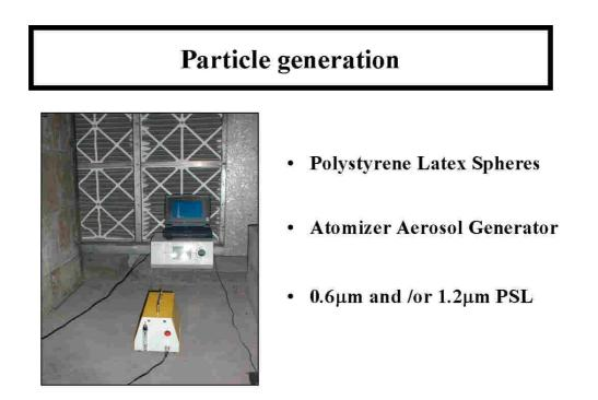
Figure 2: Generation of small monodispersed polystyrene latex spheres
