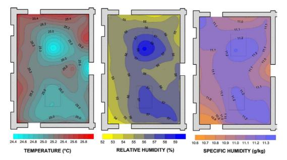
Figure 3: Effect of air conditioning with emission in the middle of the Bruegel Room, Kunsthistorisches Museum, Vienna (A). The air with different temperature and moisture content is appropriately released far from the paintings. The entrance of cooler air from the room on the right is also evident.
